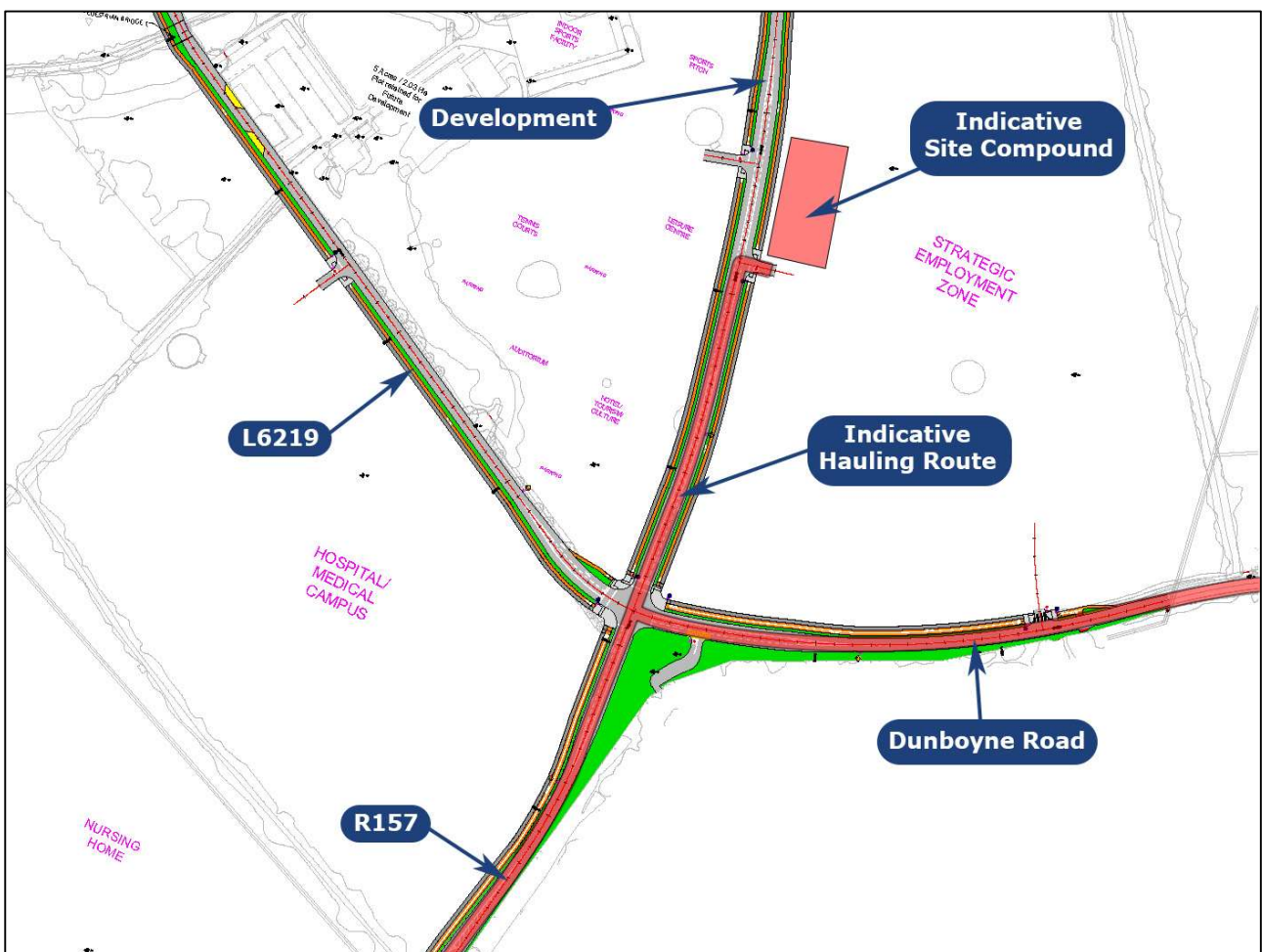
Figure 9: Indicative Site Compound and Hauling Route
